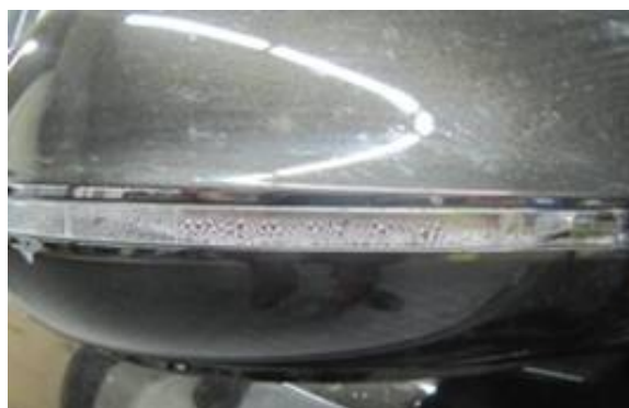
Figure 1 Condensation in turn signal lens
