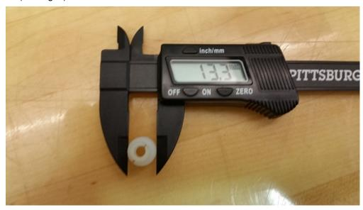
Figure 3 (Acceptable diameter after adding adhesive strip)
