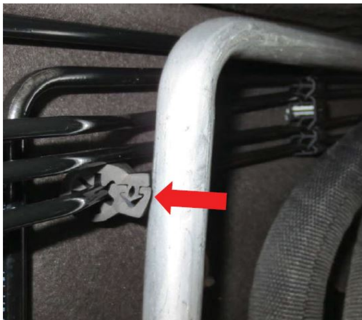
Figure 2 (example of brake line with vibration damper installed)
