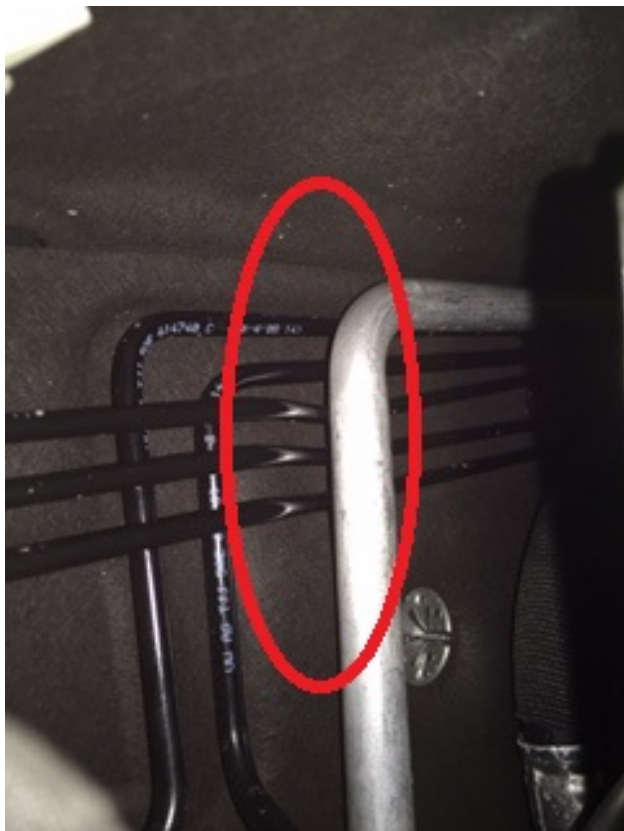
Figure 1 (contact point of refrigerant line to brake line)
