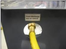
Figure 2. A flushing attachment port.
