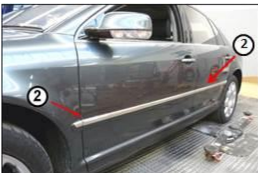
Figure 2 – Central protective strip
