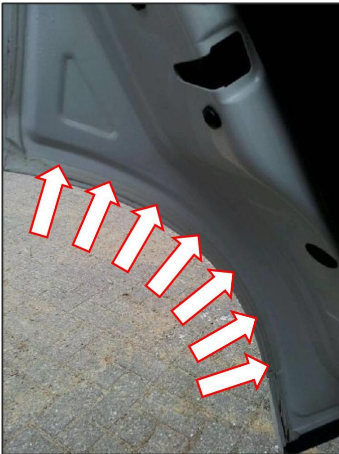
Figure 1) Arrows show the area affected by corrosion
