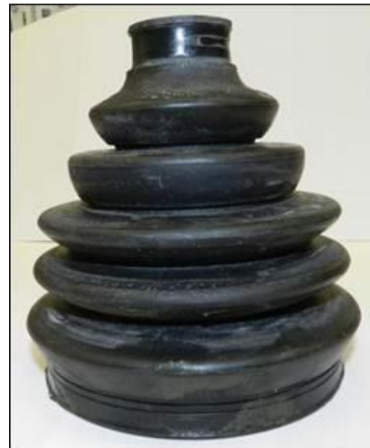
CV Boots should slide off the driveshaft after the removal of the CV Joint.
