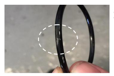
Replace the O-ring seal as necessary. Clean the Camshaft Adjustment Valve 1 -*N205*- and its connector of residual oil.
