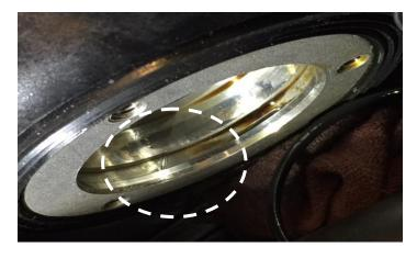
Remove the Camshaft Adjustment Valve 1 - **N205**- and its O-ring seal, inspect for nicks, cuts or irregularities in the O-ring seal.
