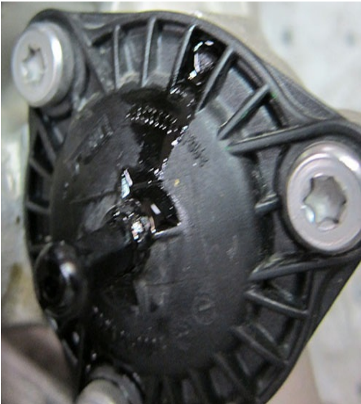
Bypass (recirculation) valve cover port broken or water/oil found inside the valve (clean the components, if necessary replace bypass (recirculation) valve assembly - released for service)
