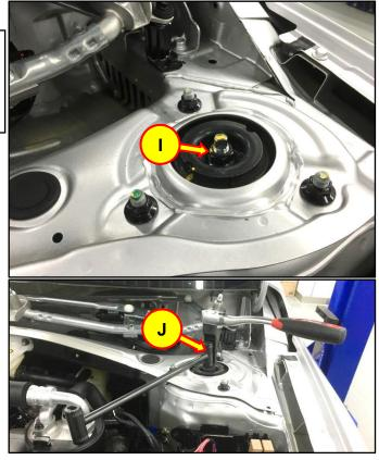
11. Install one (1) new strut nut on each side using the SST and a torque wrench.
