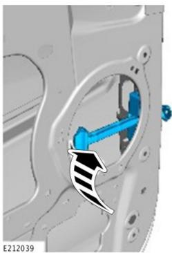
Install a replacement door check arm assembly.
