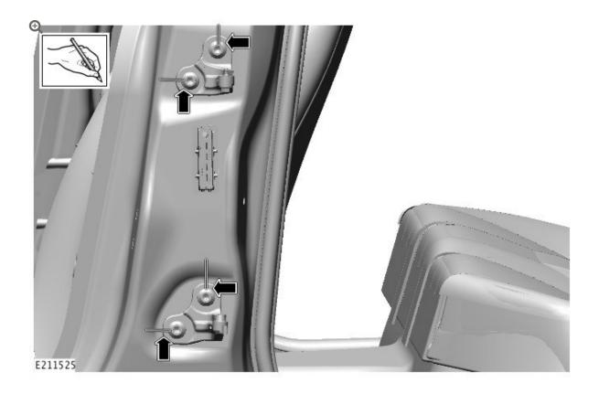
Use a non-permanent marker to mark the hinge positions against the B-Pillar as illustrated to improve alignment for installation.
