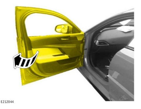
Open the door onto the hinge stops and apply pressure against the door check arm until a creak/click is heard.
