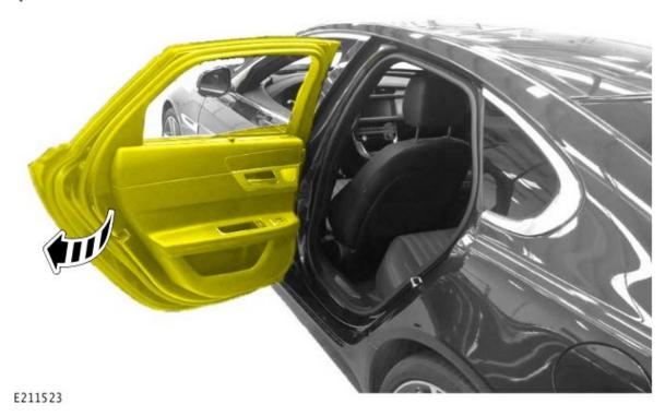
Open the rear door onto the hinge stops and apply pressure against the door check arm until a crack or click is heard.
