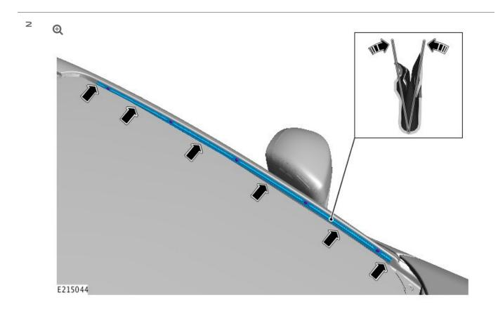
At the 6 positions shown, close the internal dimension of the windshield finisher retaining channel on the A-pillar.
