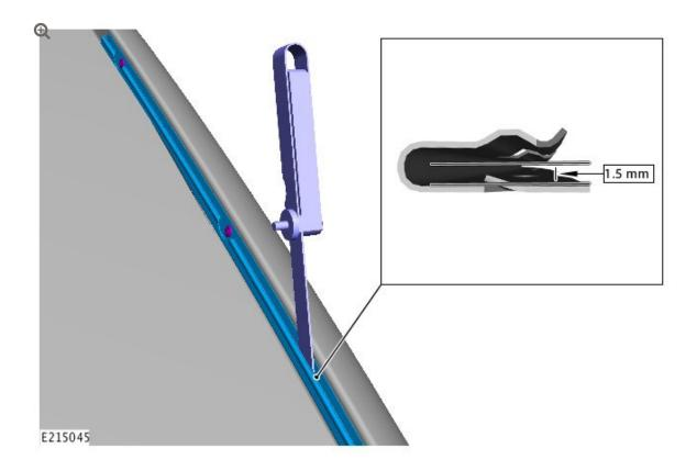
Close the windshield finisher channel to an internal dimension of 1.5 mm.
