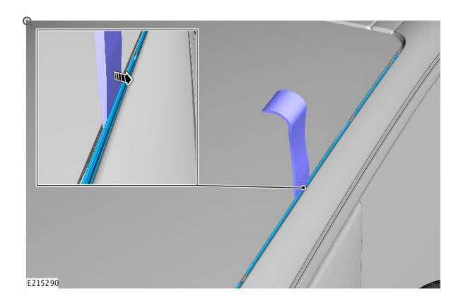
Insert a suitable, 30-40mm-wide plastic tool and pull towards the A-pillar.
