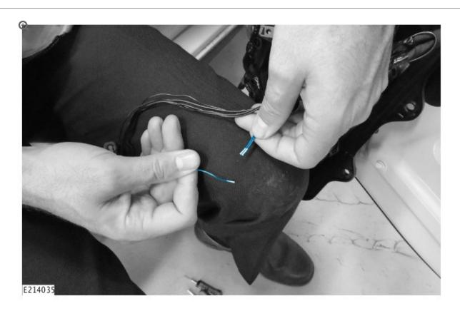
Cut the repair wire to a suitable length and prepare the front right door electrical wiring harness for a splice connector.
