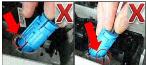
Figure 8. Incorrect installation at an angle, showing a pinched seal on the left.
