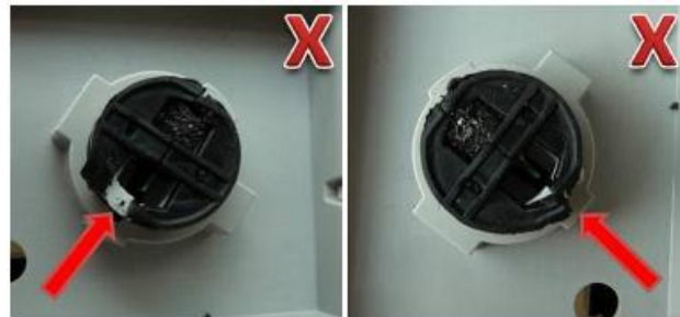
Figure 6. Examples of damaged seals
