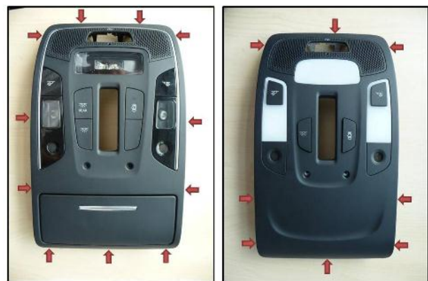
Figure 1. Clip location for A6/A7 high-line roof module (left) and for mid-line roof module (right)
