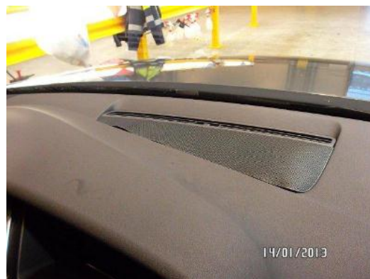
Figure 1. Deformed defroster vent trim panel.
