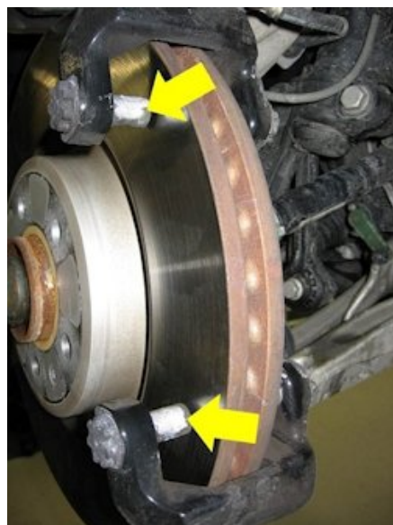
Figure 2. Caliper carrier guide pins with anti-seize ( G 052560A2 ) lubricant applied where the pads make contact.
