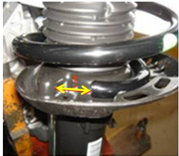
Figure 1. An incorrectly positioned coil spring.
