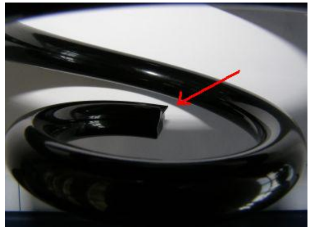
Figure 2. A burr on the end of the coil spring.
