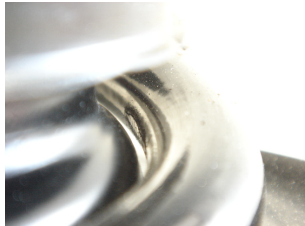
Figure 3. Abrasion on the spring retainer.
