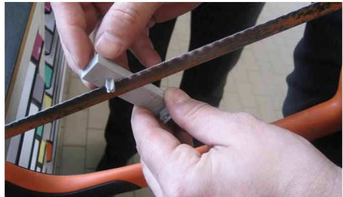
Figure 4. The zip tie with holder is installed but not tightened.
