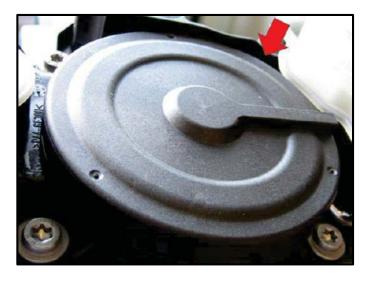
If the last retaining tab <arrow> cannot be pried open or if this is not easy, turn the cap counter-clockwise.
