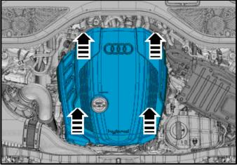
Reinstall the engine cover by positioning cover over oil filler tube and oil dipstick.
