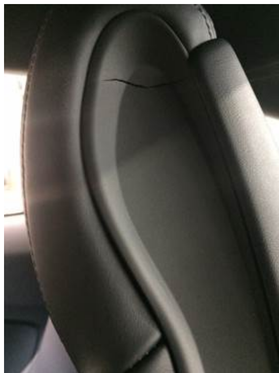
Figure 3. Front seat side trim cracked.
