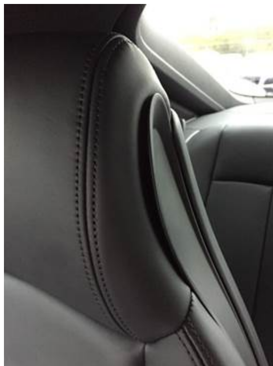
Figure 2. Inner front seat side trim loose.
