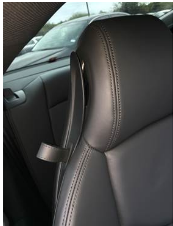
Figure 1. Outer front seat side trim loose.
