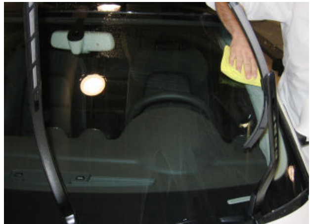
Figure 19. Dry and buff windshield.
