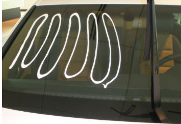
Figure 16. Cleaner applied to windshield.
