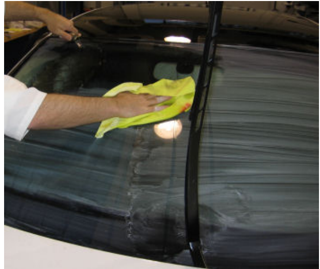
Figure 18. Rinse and wipe windshield.
