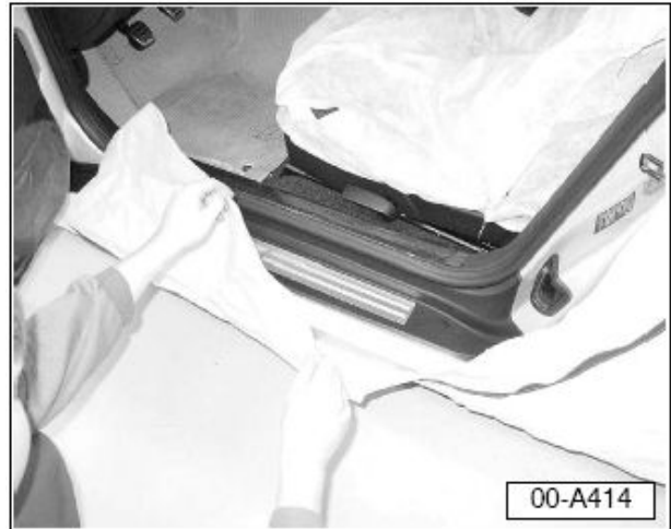
Figure 4. Remove cover from sill.
