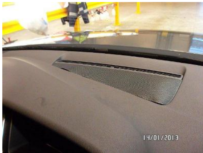
Figure 1. Deformed defroster vent trim panel.
