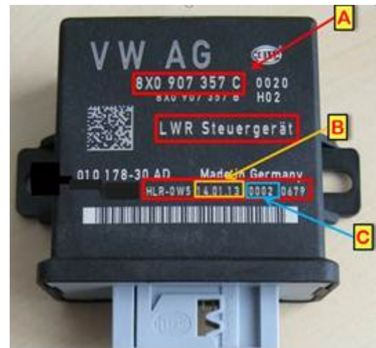
Figure 2. J745 part number (A), production date (B), production assembly line (C)
