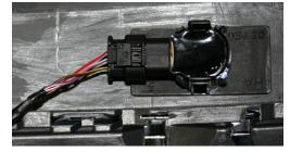
Figure 11. A sensor cable with insufficient length.
