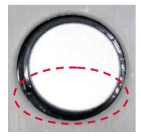
Figure 5. An incorrectly seated decoupling ring (folded).
