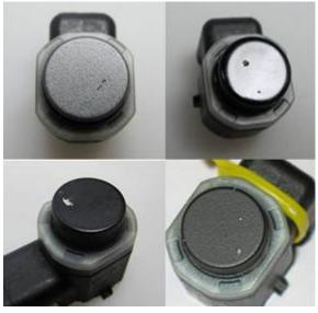
Figure 1. Stone chips causing sensor failure.
