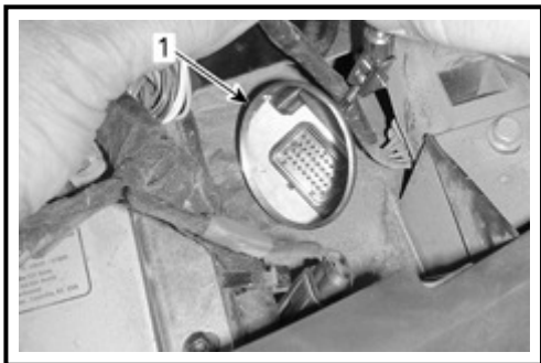
MODULE SIDE VERIFICATION USING A MIRROR
