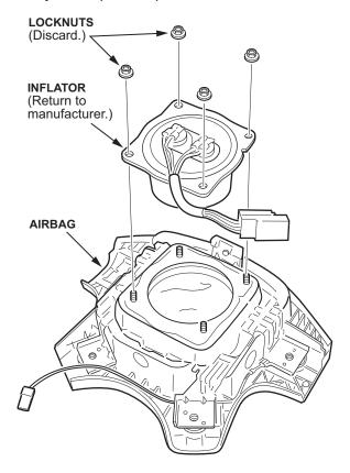
6. Use shop air to clean any debris that may be on the inflator, then remove the inflator from the airbag.
