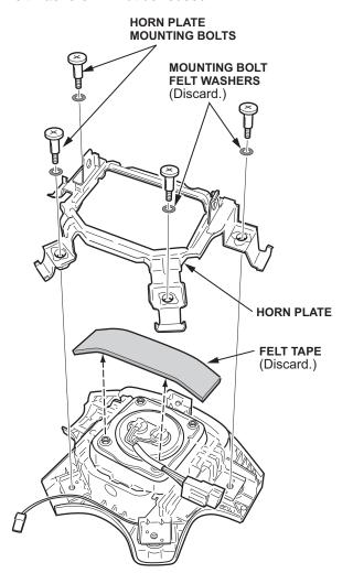
4. Remove and discard the felt tape covering the lower two inflator locknuts.
