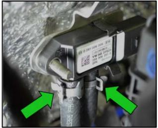
Remove the differential pressure sensor mounting nut <circle>.
