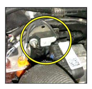
Construct the electrical connector from the differential pressure sensor <circle>.
