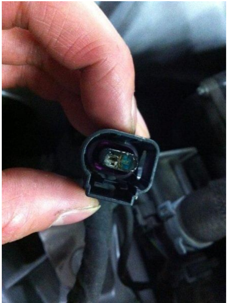
Figure 2. Corrosion formation on the connector pins.
