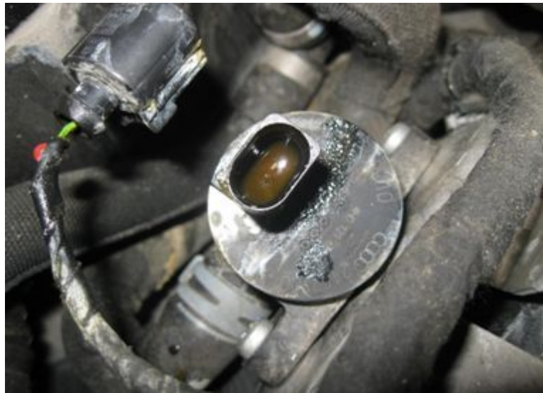
Figure 1. Coolant residue in the connector housing of the coolant regulating valve.
