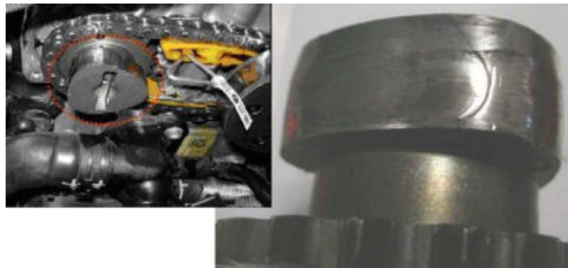
Figure 3. Excessive wear on the lobe for high pressure fuel pump in the intake camshaft.
