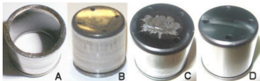
Figure 2. Cam followers in various stages of wear: holed base (A), excessive wear (B), normal wear (C), and new part (D).
