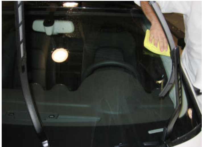
Figure 8. Drying the windshield.
