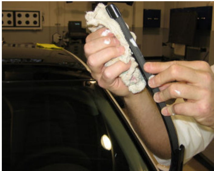
Figure 2. Cleaning wiper blades.
