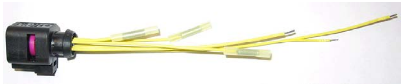
Figure 4. Crimp connectors installed on wire ends.
