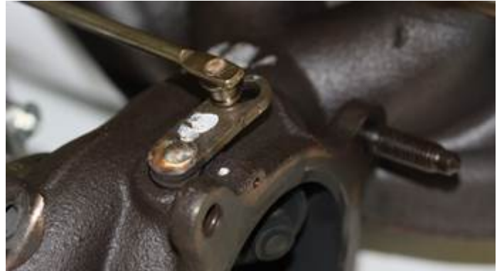
Figure 1. Disconnected wastegate linkage.
