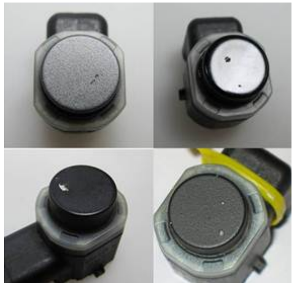
Figure 1. Stone chips causing sensor failure.
