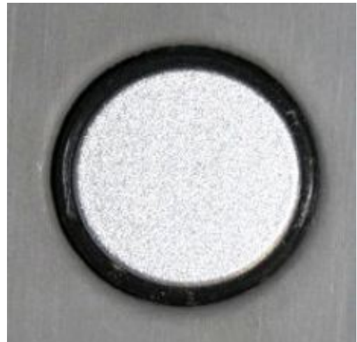
Figure 3. A correctly seated decoupling ring.
