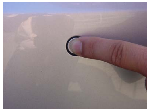
Figure 2. A pressure check on a parking aid sensor.
