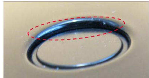
Figure 9. A recessed parking aid sensor.
