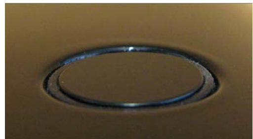
Figure 8. A correctly installed parking aid sensor.
