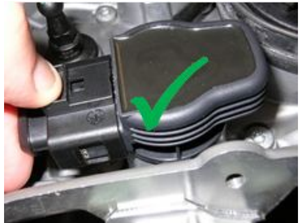
Figure 1. Correct method of disconnecting the ignition coil.
