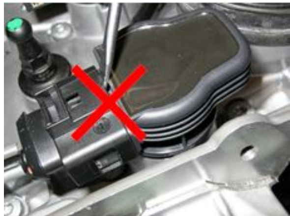
Figure 2. Incorrect method of disconnecting the ignition coil.
