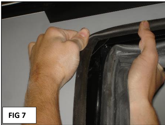
FIG 7: Press the seal firmly at the bend making sure it sticks tightly in the corner.
