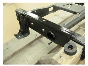
**13.** We suggest top coating the Lloyds Kryptonite with Daubert Nox-Rust® P/N X-121B "One Coat Rust Preventative Coating" (aerosol), or equivalent.
