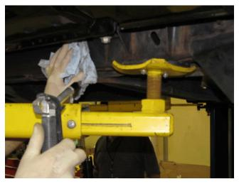
Important: The frame must be dry and free of wax/oily substances prior to application of the new coating.
