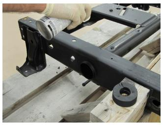
**12.** Apply a second coat of Lloyds Kryptonite. This can be a heavy coat; double and triple passes with this product, over a light first coat, are n a problem.
