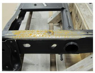
5. Using a rag and wax/grease removing solvent, remove the wax coating and any grease, oil, or undercoating from the truck frame in the affected repair area. The graphic above shows an example of a small portion of the wax coating removed.
