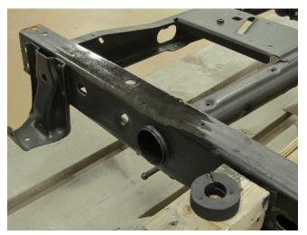
**11.** Apply a light flash-coat of Lloyds Kryptonite Metal Treatment P/N 36502 Life Long Rust Protection (14 ounce aerosol), or equivalent, to all rusted and bare areas of the frame where the wax coating was removed. This first coat should flash in approximately 3-5 minutes.
