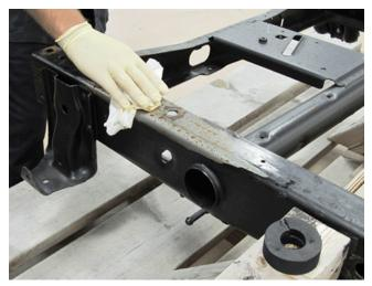
Using Lloyd's Pure Prep<sup>™</sup> Metal Surface Preparation P/N 25418 (10 fluid ounce bottle), or equivalent, saturate a towel or Scotch-Brite<sup>™</sup> (3M) pad with the pre-diluted solution and scrub the area well, rendering a foaming of the Pure Prep.<sup>™</sup> This will greatly improve adhesion a corrosion resistance in the repair areas.
