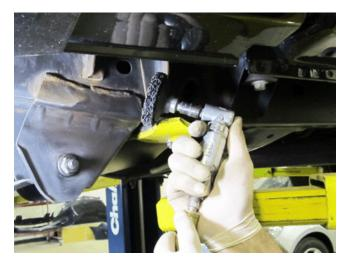
**Important:** Lloyds Kryptonite is designed to apply directly onto brown rust or clean surfaces; however any loose flakes/scale of rust need t be removed prior to application.
