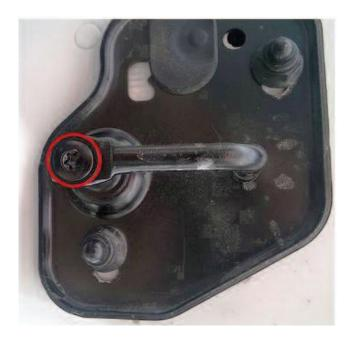
A fine adjustment to change the depth of the upper latch striker may be made at the bolt shown in the photo above.
