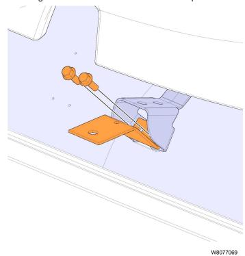
9 On the top of the center mounting bracket, install the upper sun visor stiffing bracket. Secure the bracket with a retainer.
