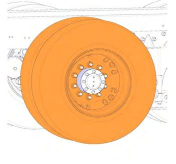
12 Install wheel/tire assembly(s). Torque wheel nuts to 610 Nm (450 ft-lb).
