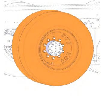
10 Install wheel/tire assembly(s). Torque wheel nuts to 610 Nm (450 ft-lb).
