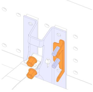
4 Install the filter on the mounting bracket.
