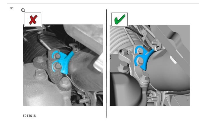
Visually inspect the Diesel Particulate Filter (DPF) bracket.
