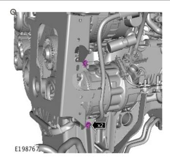
Install the charge air cooler bracket fasteners.
