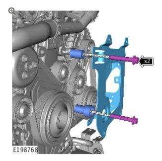
Remove the charge air cooler bracket.
