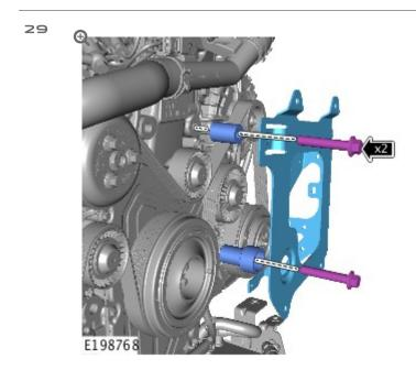
Install the charge air cooler bracket.
