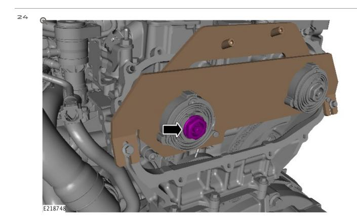
Tighten the intake camshaft VCT actuator fastener.
