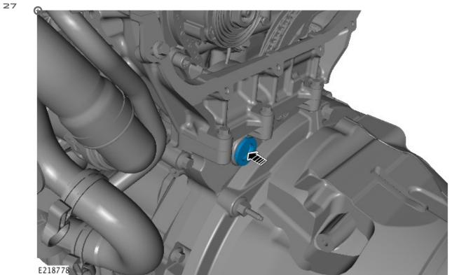
Install a new lower timing cover blanking plug.
