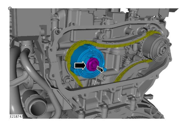
Remove and discard the intake camshaft VCT actuator.
