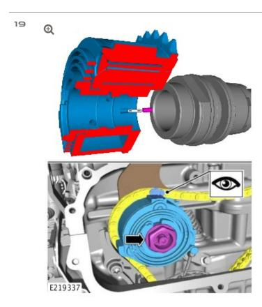
Install the new intake camshaft VCT actuator and fastener.
