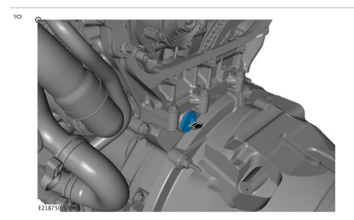
Use a suitable tool to remove the lower timing cover blanking plug.
