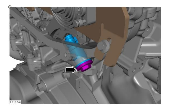
Install the upper timing chain tensioner.
