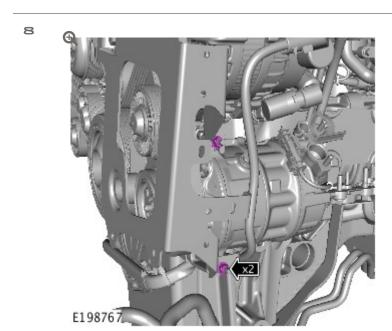
Remove the charge air cooler bracket fasteners.
