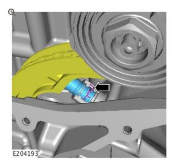
Release the upper timing chain tensioner piston.
