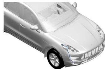
Installation position of breather hose
