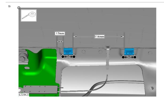
Adjust the position of the new tailgate clips as shown.
