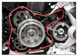
2) Install the **generator cover (21)** within 5 minutes of applying the sealant and drive it fully home on the crankcase.
