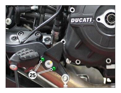
15) Install the **special tool Part no.887131749** by tightening the 2 screws to a torque of <u>5 Nm ± 10%</u> and remove the generator cover.
