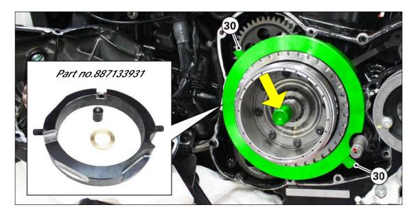
21) Using a sliding arm puller remove the driven gear, flange, starter clutch, flywheel and rotor assembly.
