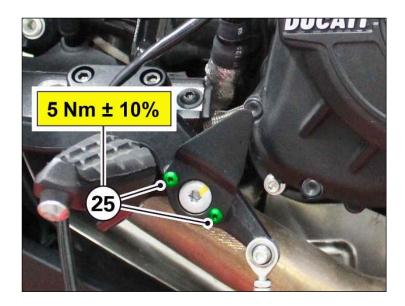
10) Release clutch slave cylinder, engine rpm sensor and gear sensor from the elastic band.
