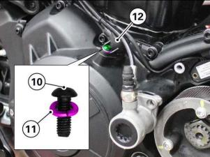
7) Move the gear sensor, the clutch slave cylinder and the engine rpm sensor away from the working area, tying them with an elastic band as shown in the figure.
