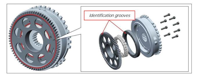
3) Fix old rotor (35) on the flywheel assembly of kit Part no. 69928312A orienting it so that the hole (36) of the rotor is aligned with the engraved point (37) of the flywheel, as shown in the figure.
