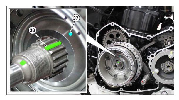
3) Insert the copper washer supplied with special tool Part no. 887133931 on the crankshaft. <u>The copper washer must be used ONLY to insert the flywheel completely on the crankshaft and be</u>
