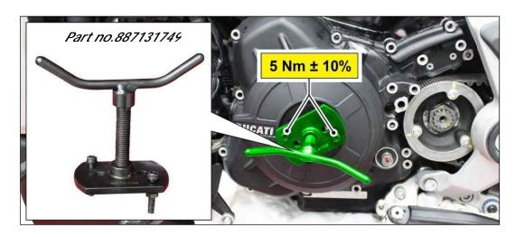
16) Remove special tool Part no.887131749.
