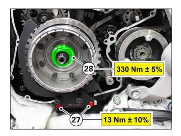
• remove nut (28) and copper washer;
