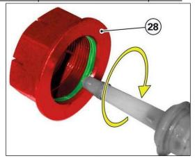
Perform the final tightening of **nut (28)** to a torque of <u>330 Nm ± 5%</u>.
