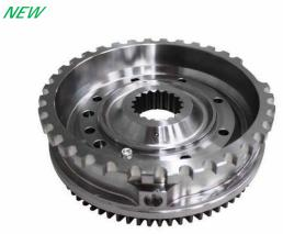
Below is the correct orientation of the flywheel assembly present in kit Part no.69928312A.
