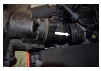
Reinstall air duct hose in the direction of the <arrow> and reinstall the clamp.
