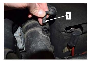
Reinstall low pressure hose <1> from air filter housing.
