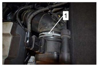
• Loosen clamp <3> to remove air duct hose.
