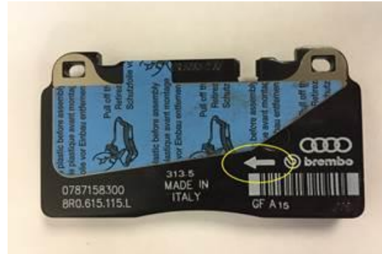
Figure 2. Directional arrow on the back of front brake pad.
