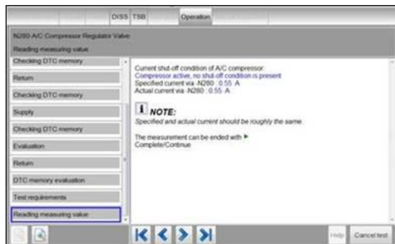
Figure 5. Checking N280 signal value Measuring Value Block.
