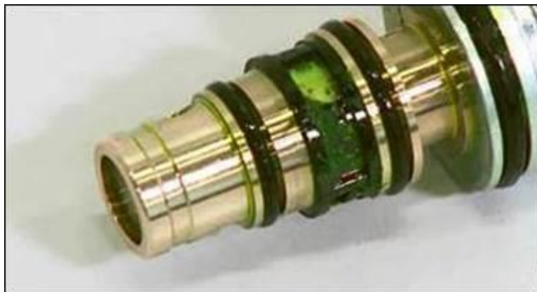
Figure 15: Severe contamination at the N280 valve filter screen.
