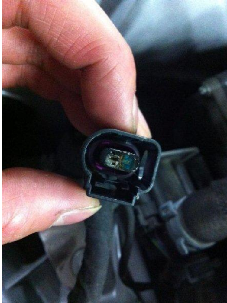
Figure 2. Corrosion formation on the connector pins.
